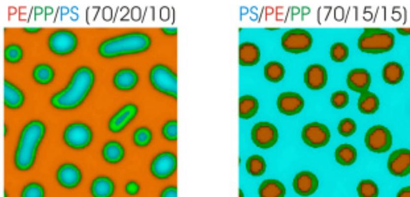
In the case that polyethylene or polystyrene is major part, the minor components make the core-shell structure like the previous figure.
