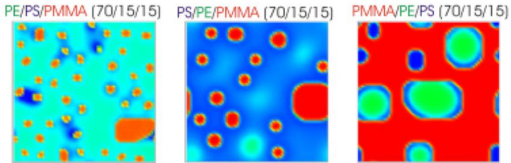
In the case that polyethylene or poly (methyl methacrylate) is major part, the minor components make the core-shell structure. In the other case where polystyrene is major part, the minor components make separated droplet.
