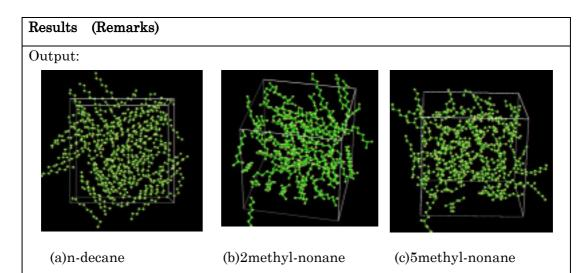
Fig.1 The snapshots of the different chains systems at 11 nano seconds after quenching to 180K from 420K. The n-decane chains (a) show ordered structure and create several of crystal domains. On the other hand, 2methyl-nonane chains (b) made the partial ordered conformations, but most of chains are still random.5methyl-nonane chains (c) have no ordering structures.
