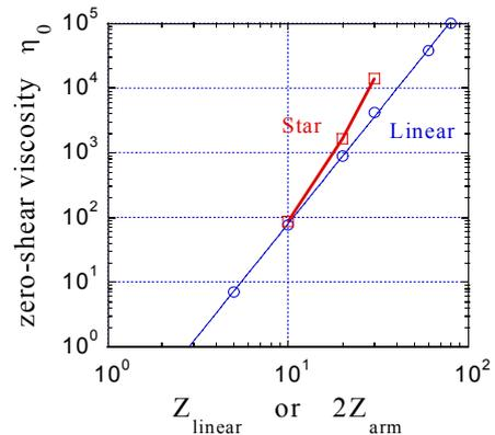
Fig.2 Molecular weight ( $Z$  or  $Z_a$ ) dependency of the zero shear viscosity.
